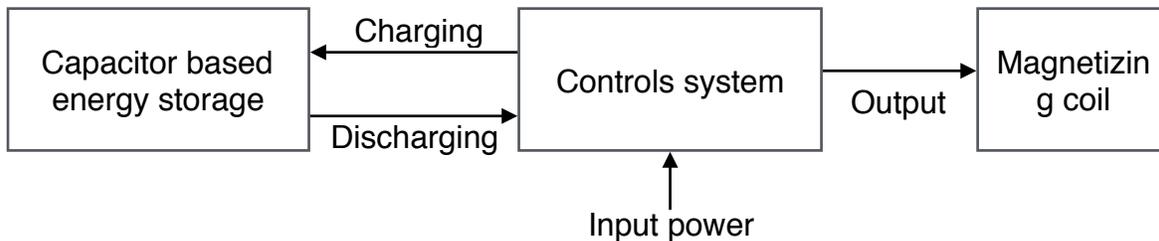
**Figure 1:** a block diagram of the proposed system. A capacitor-based storage system provides safety benefits over other possible storage systems, and the controls automates the system to make it cost-effective and easy to use.
