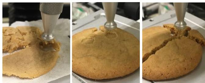
**Figure 4:** Texture Analyzer measuring Baking Time Cookies, from left to right: 6min, 10min, and 14min
