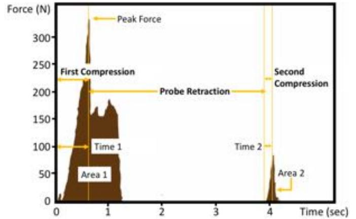
**Figure 1:** Texture Profile Analysis (TPA) Data from Trial of 14 Min Cookies
